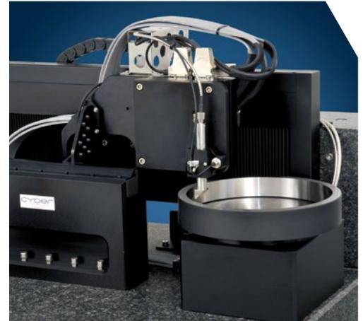
Roughness measurement on an engine part
